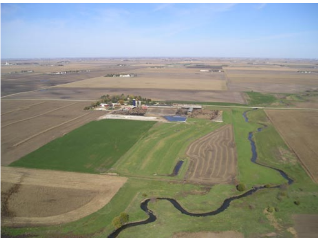
Aerial of overall VTA system after completion. Crops are now grown east of the VTA channels in what used to be an unusable swamp. The stream is protected.
